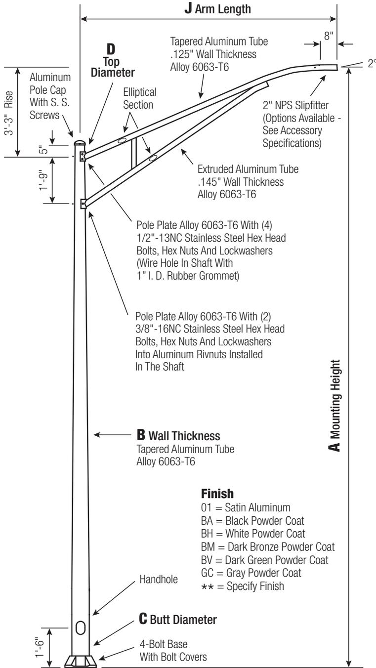
**WARNING:** Do not install light pole without luminaire. *Satin Aluminum or Powder Coated Finish per Customer Specification.*
