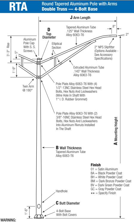
Do not install light pole without luminaire.
