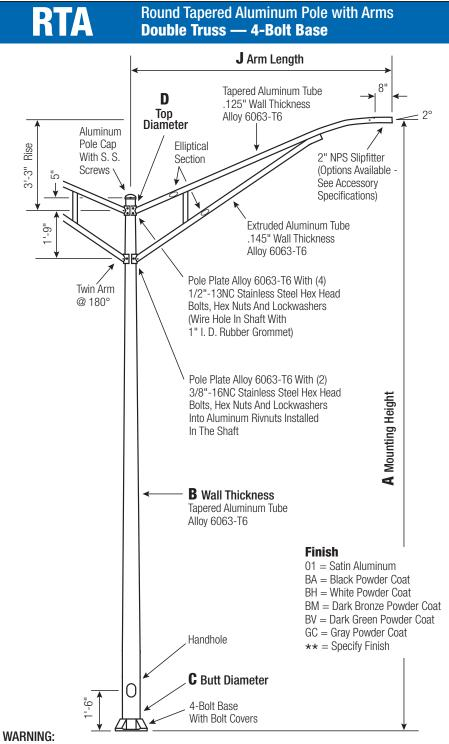
Do not install light pole without luminaire.
