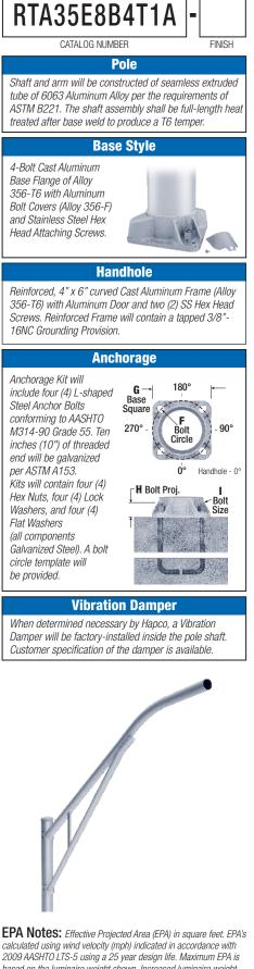
calculated using wind velocity (mph) indicated in accordance with 2009 AASHTO LTS-5 using a 25 year design life. Maximum EPA is based on the luminaire weight shown. Increased luminaire weight may reduce the maximum EPA. If weight is exceeded, or if other design life or code is required, please consult the factory
