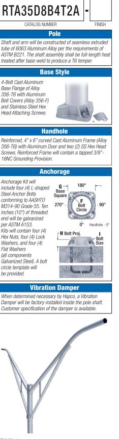
**EPA Notes:** Effective Projected Area (EPA) in square feet. EPA's calculated using wind velocity (mph) indicated in accordance with 2009 AASHTO LTS-5 using a 25 year design life. Maximum EPA is based on the luminaire weight shown. Increased luminaire weight may reduce the maximum EPA. If weight is exceeded, or if other design life or code is required, please consult the factory.
