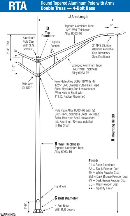
Do not install light pole without luminaire.
