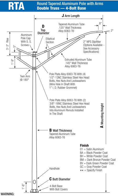
Do not install light pole without luminaire.
