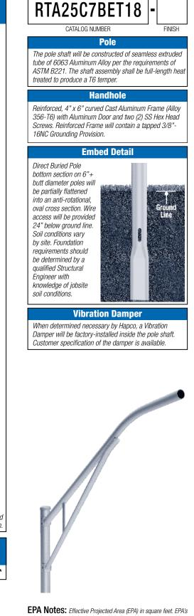
EPA Notes: Effective Projected Area (EPA) in square feet. EPA's calculated using wind velocity (mph) indicated in accordance with 2009 AASHTO LTS-5 using a 25 year design life. Maximum EPA is based on the luminaire weight shown. Increased luminaire weight may reduce the maximum EPA. If weight is exceeded, or if other design life or code is required, please consult the factory.
