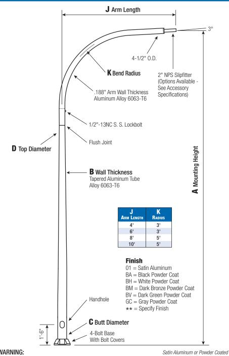
include four (4) L-shaped Steel Anchor Bolts conforming to AASHTO 270° M314-90 Grade 55. Ten inches (10") of threaded end will be galvanized per ASTM A153. Kits will contain four (4) Hex Nuts, four (4) Lock Washers, and four (4) Flat Washers (all components Galvanized Steel). A bolt circle template will be provided.
