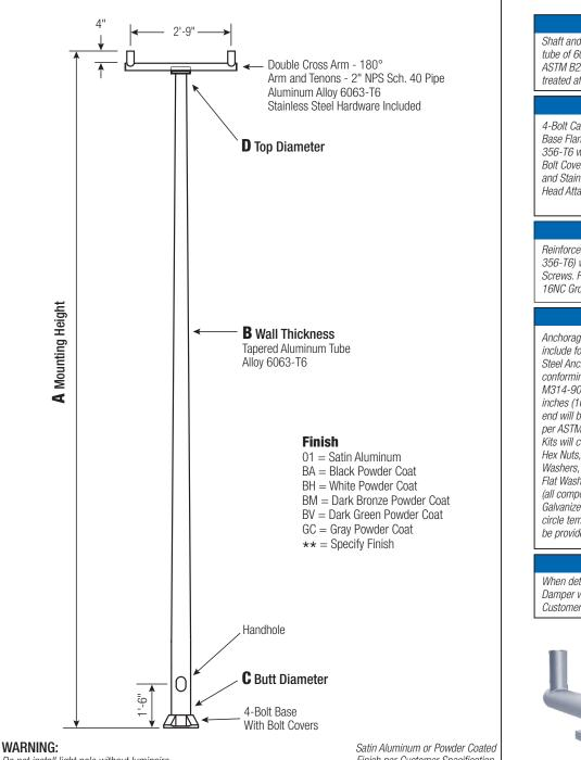
Do not install light pole without luminaire.
