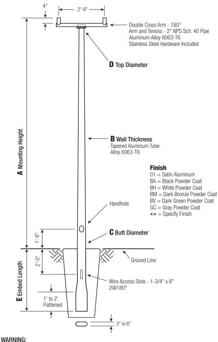
Do not install light pole without luminaire.
