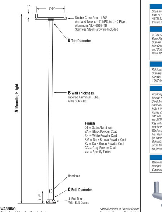
Do not install light pole without luminaire.
