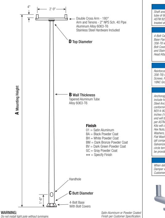
C B A WALL Mtg. BUTT Махімим ЕРА LUM. DIAMETER THICKNESS 90 100 120 130 **CATALOG NUMBER** HGT. WEIGHT 110 0.188" 40 10 60 7.6 5.8 5.4 4.2 3.4 RTA40D1C4F20-\*\* C D G H П BOLT CIR. DIA. BASE SQ. BOLT PROJ. BOLT SIZE BUTT DIA TOP DIA 1 x 48 x 4 10 6 14 - 15 14 3.25
