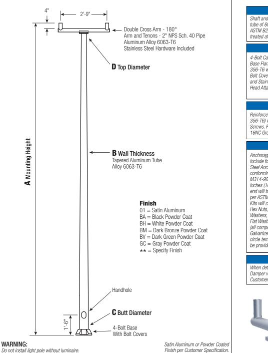
C B A WALL Mtg. BUTT Махімим ЕРА LUM. DIAMETER THICKNESS 90 100 120 130 **CATALOG NUMBER** HGT. WEIGHT 110 0.188" 35 8 30 5.2 3.6 3.2 2.4 1.8 RTA35D8B4F20-\*\* C G H D П BOLT CIR. DIA. BASE SQ. BOLT PROJ. BOLT SIZE BUTT DIA TOP DIA 8 4.5 11 - 12 11.25 2.75 1 x 36 x 4
