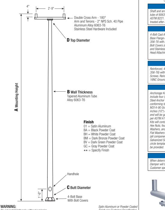
Do not install light pole without luminaire.
