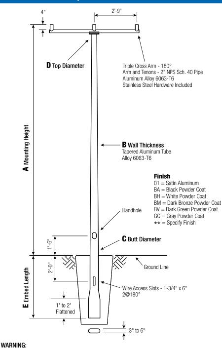
Do not install light pole without luminaire.
