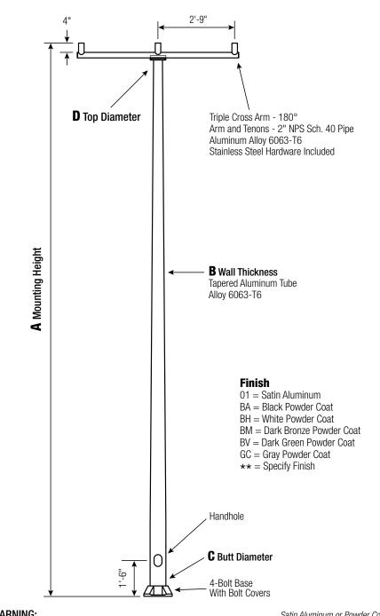
Pole Shaft and arm will be constructed of seamless extruded tube of 6063 Aluminum Alloy per the requirements of ASTM B221. The shaft assembly shall be full-length heat treated after base weld to produce a T6 temper. Base Style 4-Bolt Cast Aluminum Base Flange of Alloy
