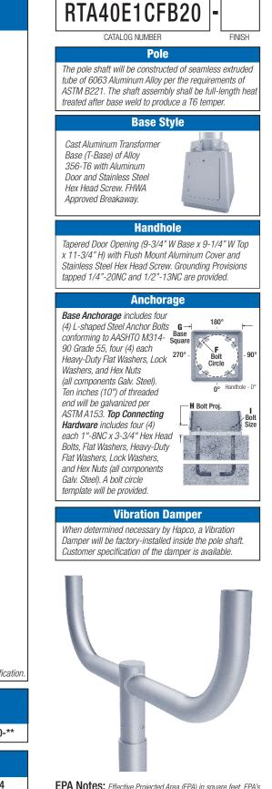
EPA Notes: Effective Projected Area (EPA) in square feet. EPA's calculated using wind velocity (mph) indicated in accordance with 2009 AASHTO LTS-5 using a 25 year design life. Maximum EPA is based on the luminaire weight shown. Increased luminaire weight may reduce the maximum EPA. If weight is exceeded, or if other design life or code is required, please consult the factory.
