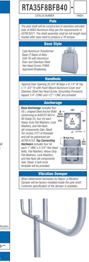
**EPA Notes:** Effective Projected Area (EPA) in square feet. EPA's calculated using wind velocity (mph) indicated in accordance with 2009 AASHTO LTS-5 using a 25 year design life. Maximum EPA is based on the luminaire weight shown. Increased luminaire weight may reduce the maximum EPA. If weight is exceeded, or if other design life or code is required, please consult the factory.
