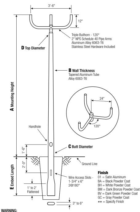
Do not install light pole without luminaire.
