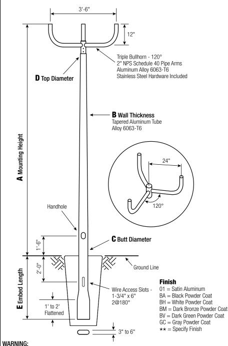
Do not install light pole without luminaire.
