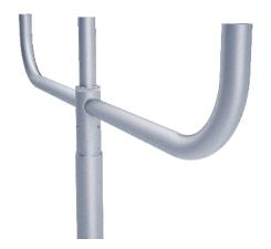
EPA Notes: Effective Projected Area (EPA) in square feet. EPA's calculated using wind velocity (mph) indicated in accordance with 2009 AASHTO LTS-5 using a 25 year design life. Maximum EPA is based on the luminaire weight shown. Increased luminaire weight may reduce the maximum EPA. If weight is exceeded, or if other design life or code is required, please consult the factory.
