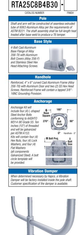
EPA Notes: Effective Projected Area (EPA) in square feet. EPA's calculated using wind velocity (mph) indicated in accordance with 2009 AASHTO LTS-5 using a 25 year design life. Maximum EPA is based on the luminaire weight shown. Increased luminaire weight may reduce the maximum EPA. If weight is exceeded, or if other design life or code is required, please consult the factory
