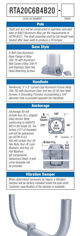
calculated using wind velocity (mph) indicated in accordance with 2009 AASHTO LTS-5 using a 25 year design life. Maximum EPA is based on the luminaire weight shown. Increased luminaire weight may reduce the maximum EPA. If weight is exceeded, or if other design life or code is required, please consult the factory.
