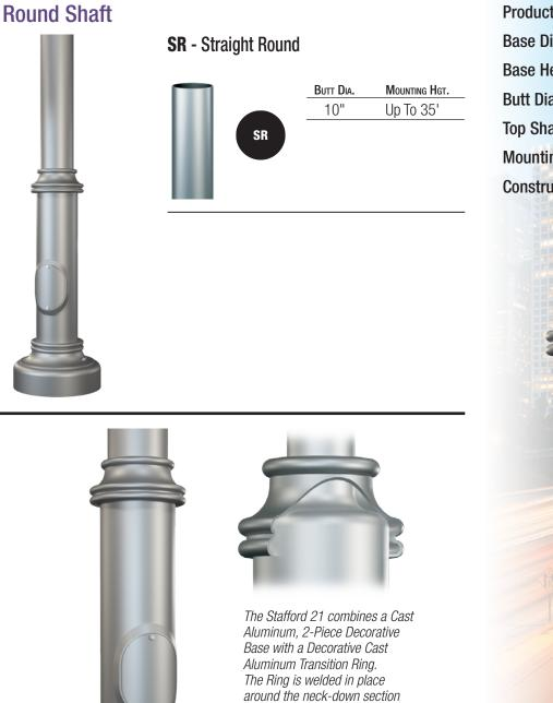
of the pole shaft, allowing designers to customize Base Heights. Product Code: S16 Base Diameter: 21" Base Height: 4'-0" Butt Diameter: 10" Top Shaft Diameter: 6" Mounting Heights: Up to 35' Construction: Aluminum Alloy 356
