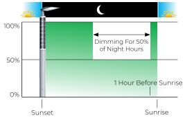
Custom: Fully Customizable Profiles Can Be Specified To Meet Building Efficiency Codes
