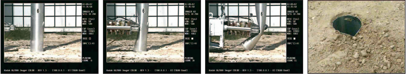
Screen captures of high speed video of Hapco's Direct Buried FHWA accepted Breakaway Aluminum Pole.
